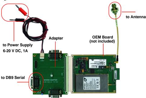
Figure 2-1. OEM board connected to Evaluation Kit
